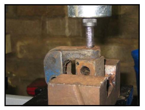
It is likely that the pins removed from the joint will not be suitable for re-use due to wear or corrosion. New pins can be made from "engineer's" dowels which are precision ground, case hardened steel pins. They can be cut and shaped with a grinder by a competent person. Care should be taken not to overheat them as this can change the temper of the metal and affect wear and durability.
