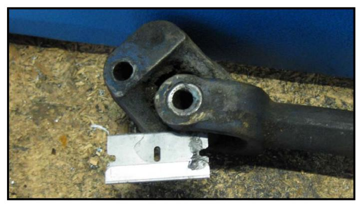
Once the plastic has been cut or broken the block can be withdrawn from the yoke on the shaft. The broken bearing (or bearings) can be removed from the yoke by pressing into the centre of the yoke.
