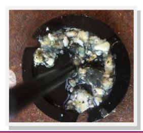
There are 2 filter screens supplied a fine & coarse one this is the fine one you can see that it works & prevents the rubbish before entering the radiator
