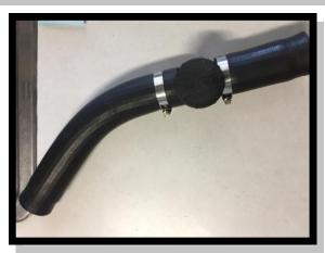
This is a In-Line Radiator filter it's a good thing to have especially if you have had the radiator re-conditioned or flushed also think about a new radiator cap & hi flow thermostat.
