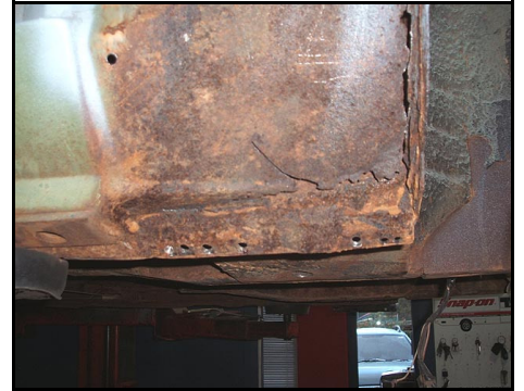
Rusted inner sill panel (underneath lower front guard RHF)
