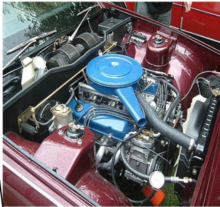
Modified 4.4 EFI V8. Details in covering article
