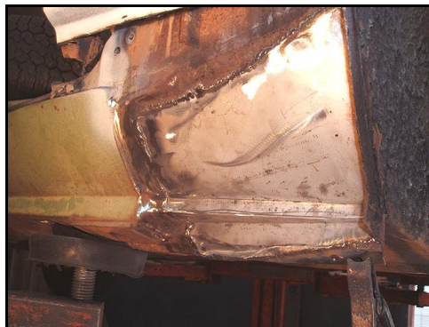
New inner sill panel welded in place (Note all welding is to be ground back so as to look good)
