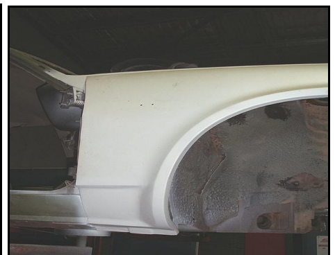
Lower guard section repaired & welded back on
