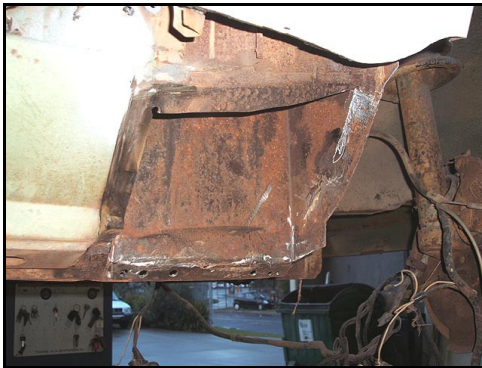
Inner sill panel cut out. Note "cut off" lower front guard
