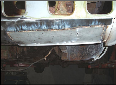
Damaged/rusted section of stone tray replaced.
