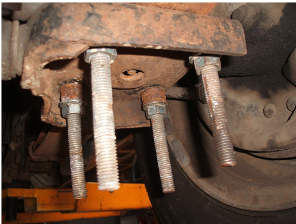
A shot of the "U Bolts" after the lowering blocks were taken out...Love the washers huh!
