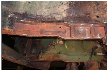
Rail with rust cut out (Note Tubes)
