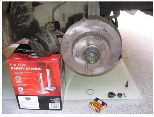
Re-fit the Spring Ring removed from the Old Oil Seal earlier, if you are reusing it, and install the New or Old Seal over the Inner Wheel Bearing, Flat Side Outwards. Tap it in softly with a Wooden Block and Hammer.
