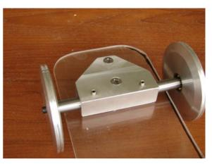
On the right is the front axle which can be adjusted to enable the Racer to run straight.
