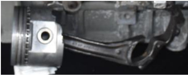
Piston number 5 & rod – both bolts still intact! ... . Number 5 – missing entire big end.
