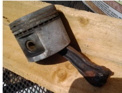
Piston number 5 & rod – both bolts still intact! ... . Number 5 – missing entire big end.
