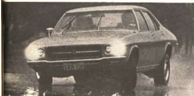
THE Holden understeers (even in the wet) with moderate body roll, and final plough understeer. There is some evidence of front end knee and a little tyre distortion, but generally handling is "safe".
