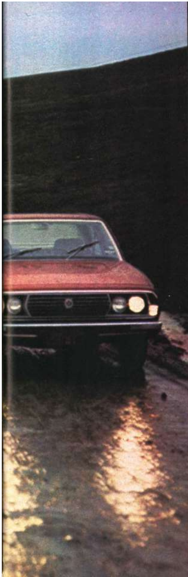
OVERSTEER. Leyland's P76 wallowed through the mud in our tough wet-weather rough-roads test. Optional oversteer was available but low-g geared steering reduced manoeuvrability.
