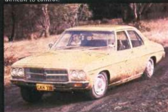
UNDERSTEER. GM's Holden charged straight on regardless, only displayed oversteer when excessive power was deliberately applied. Steering offered more precise control than others, but front end plough was often heavy.
