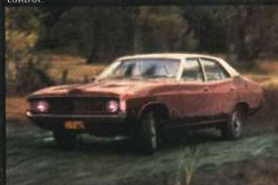
OVERSTEER. Ford's Falcon was predominantly and predictably an oversteerer under virtually every condition. Transition from the neutral stance was sometimes rapid, difficult to control.
