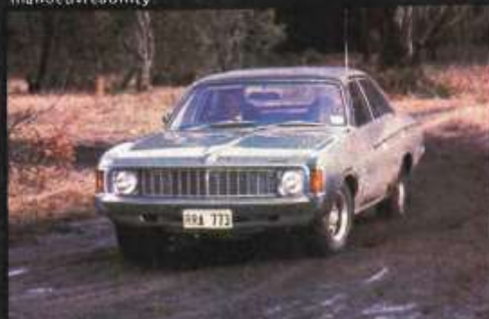
UNDERSTEER. Chrysler's Ranger ploughed straight ahead on its fin rims, but switched rapidly to oversteer when power was applied. Low-g geared steering also reduced control.
