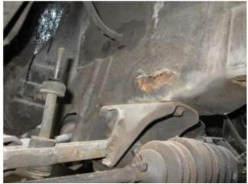
Let the rust repairs commence, with work and other commitments progress on the rust repairs have been slow but with a new rust repair section for the left sub frame rail sourced from
