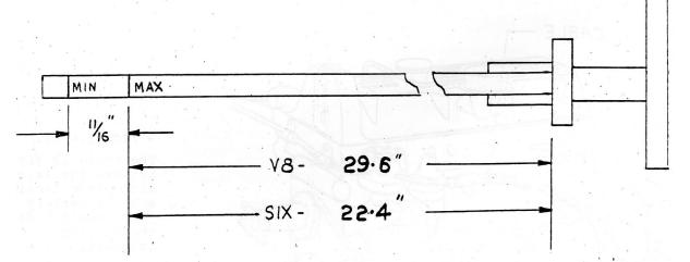
It is also of the UTMOST IMPORTANCE that the transmission be topped up to the correct level before being returned For this purpose the dipstick can be remarked, to owner. but only as a temporary measure pending replacement.
